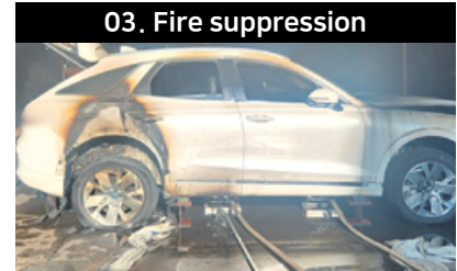
Direct Cooling-down of Battery Cells & Preventing Reignition
