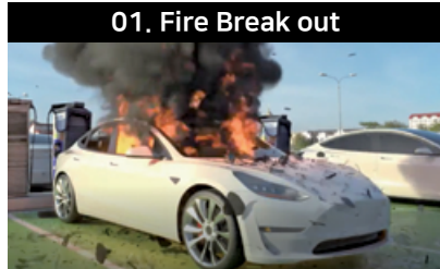
Thermal runaway of battery(800°C)
