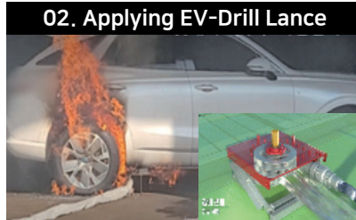
Penetrating Battery Case & Supplying Fire Water
